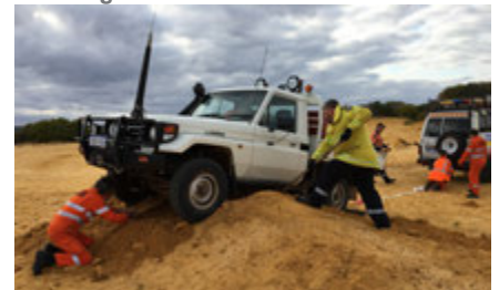
“Resting” the front axel on sand
