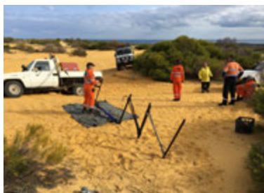
Three point anchor for a safe recovery
